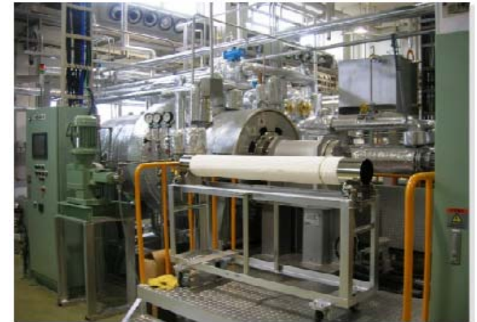
Fig.12 Practical supercritical fluid plant having 350 litter treating bath for fiber and textile treatments.
