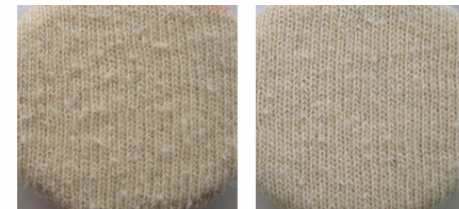
Figure 6. Knitted wool fabrics untreated (left, grade 1) and plasma coated (right, grade 2) at 5000 rubs.
