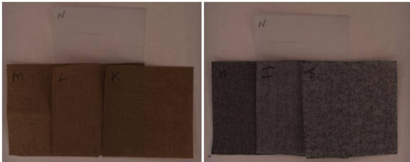
Figure 2. Photographs of cotton fabric impregnated with CuO NPs via the ‘in situ’ method (LHS) and the ‘TTS’ method (RHS)
